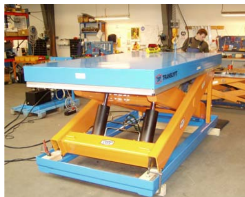
TRANSLYFT explosion proof lifting table for Borealis, Norway during production
